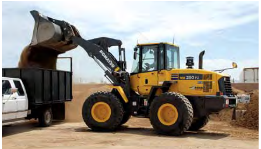
Pioneer Landscaping Materials likes the versatility its Komatsu parallel tool carriers offer. This WA250PZ-6 has a quick coupler for fast attachment changes from its specialty attachment for carrying boulders to a bucket for load-and-carry applications.
